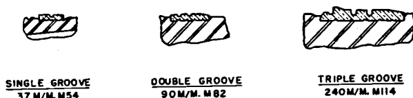
FIG. 40. Types of rotating bands for artillery projectiles.
