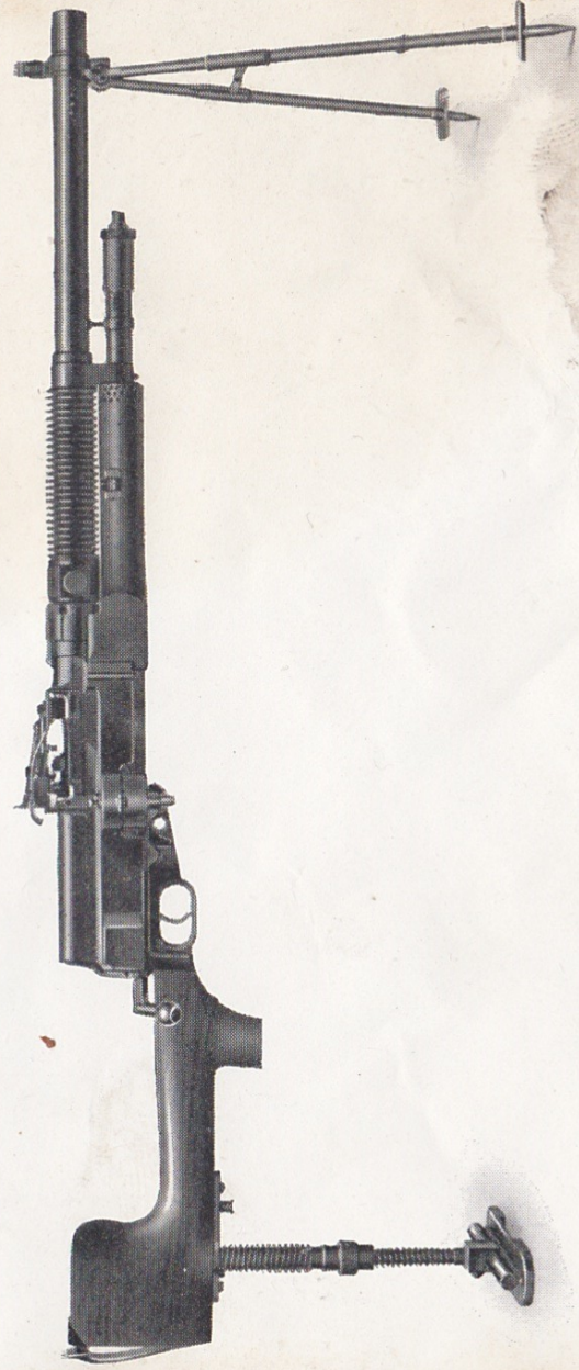
Infantry model with elevating gear. PLATE I.
