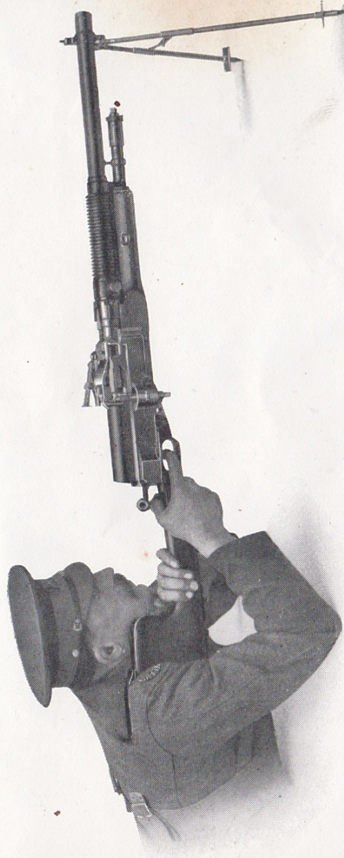
FIG. 13.—Firing position without elevating gear; shoulder strap opened and pressed down firmly against shoulder, left hand grasping stock.
