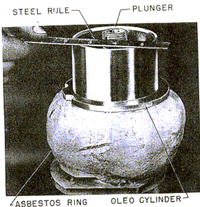
Figure 124—Checking Cotter Pin Hole Location
