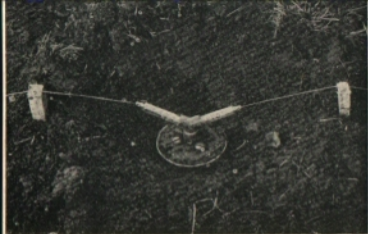
German "S" mine with "Y" adapter and two pull igniters shown uncovered.
